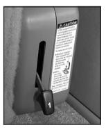
Pull up on the release lever labeled 1 located on the rear of the seatback and push the seatback forward.
